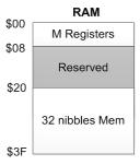
In addition to the immediate addressing mode, the indexed addressing mode is also supported. The page and address of the indexed RAM should be stored into RPT1 and RPT0 first, and users can read from or write in the XMD memory register to realize the indexed RAM access.
